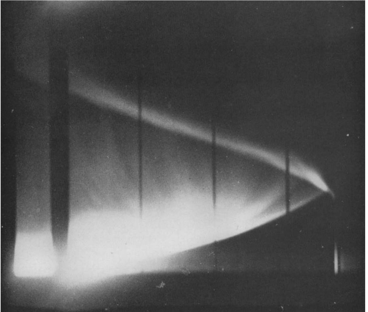
Figure 2. This photograph shows a shock reflected from a metal slug. At the reflecting surface the incident Mach number is 11.1, and p_1 \tau = 0.56 , in units of cm of mercury times microseconds.
